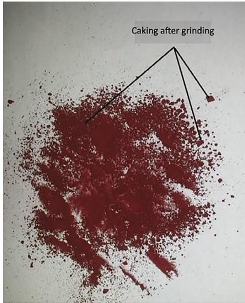
Fig. 6. Caked material after the vertical ball mill grinding.
