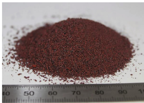
Fig. 1. Bulk image of the \alpha -Fe 2 O 3 red powder.
