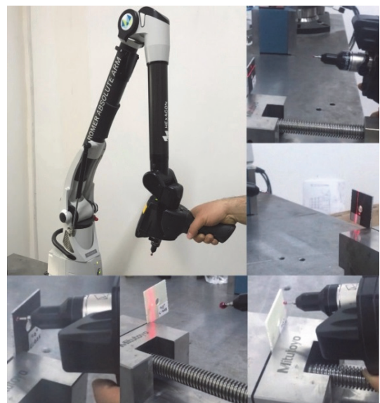
Figure 5 Dimensional control by the line laser scanner
