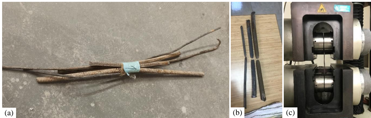
Figure 6: (a) Reinforcement taken from a collapsed buildings' column, (b) tested reinforcement, (c) tension test of a rebar.
