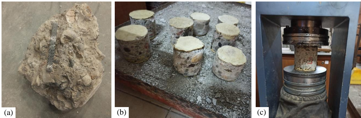
Figure 5: (a) A large piece of concrete and (b) core samples, (c) concrete compression test.
