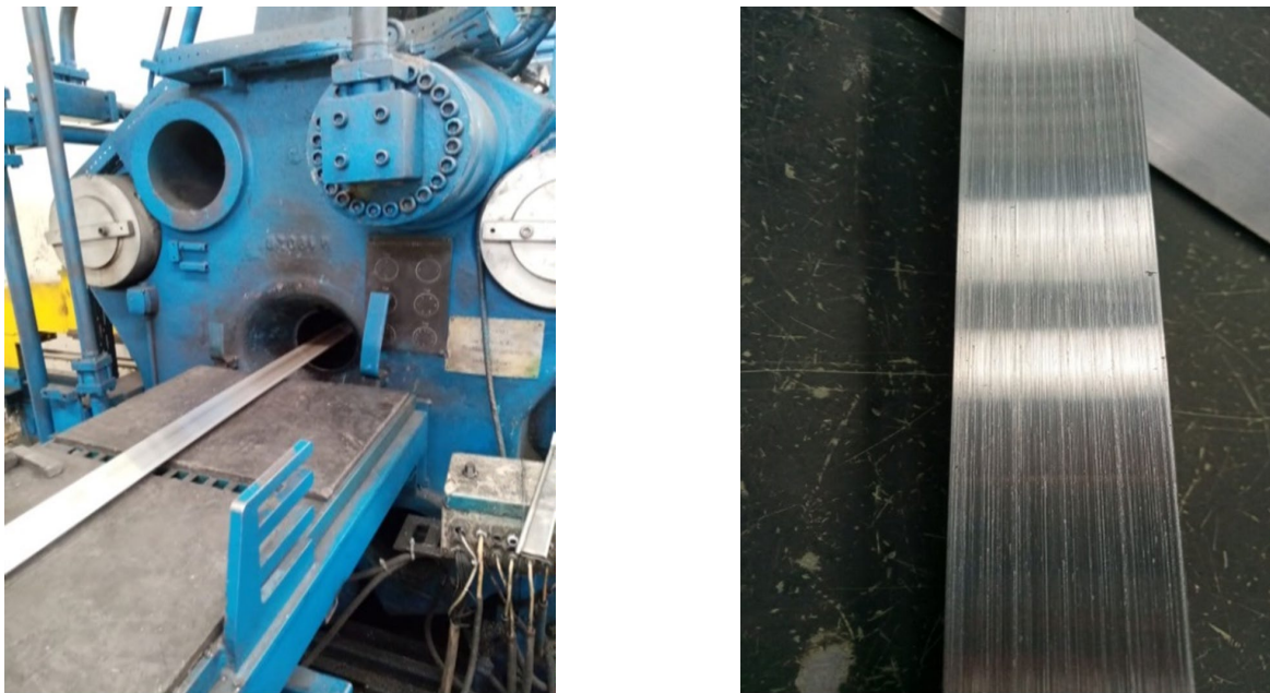
FIGURE 9. Extrusion process of AA6060 Alloy and magnified surface view of the extruded product.
