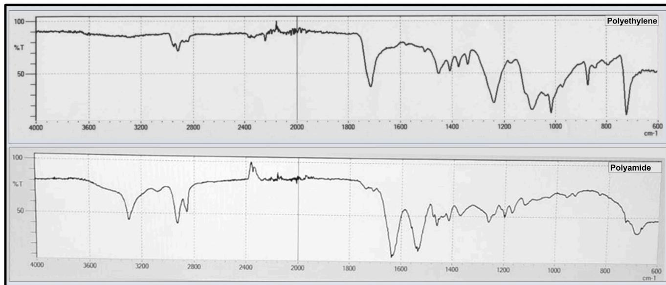
Fig. 5. Representative FTIR spectra for major identified polymers.
