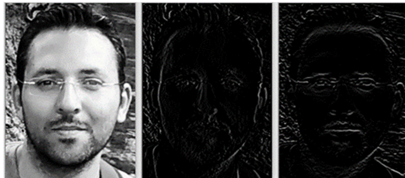
Figure 2. Original image (left), gradient image on x -axis (center), gradient image on y -axis (right).
