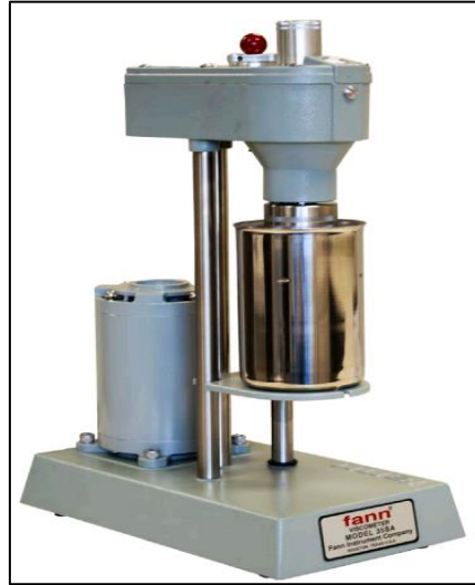
Şekil 3.5. Fann Model 35 viskozimetre (Fann-Manuel, 2016).
