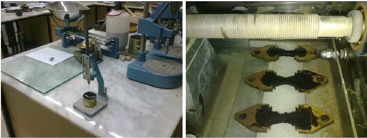
Fig. 4 Testing of penetration and ductility testing of modified bitumen samples
