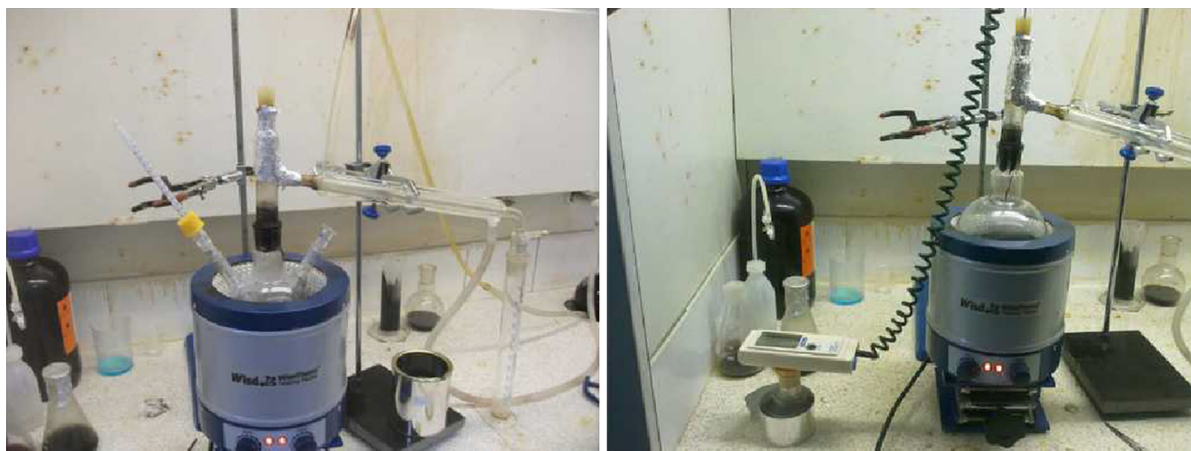
Fig. 2 Prototype pyrolysis units for preparation of modified bitumen samples in laboratory conditions
