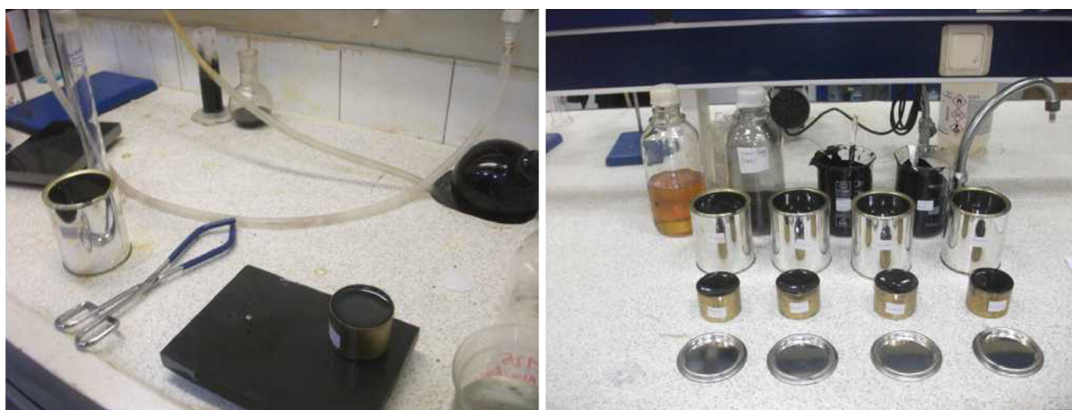
Fig. 3 Samples preparation of modified bitumen for density, penetration, ductility, softening–heating–flash points and resolution testing
